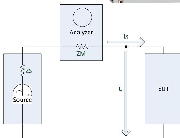
Fig. 1: Measurement setup acc. IEC/EN 61000-3-2
