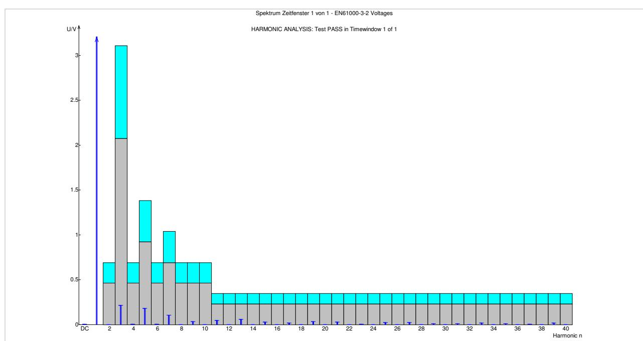
Fig. 7: Frequency spectrum of the voltage source (PAS 5000)
