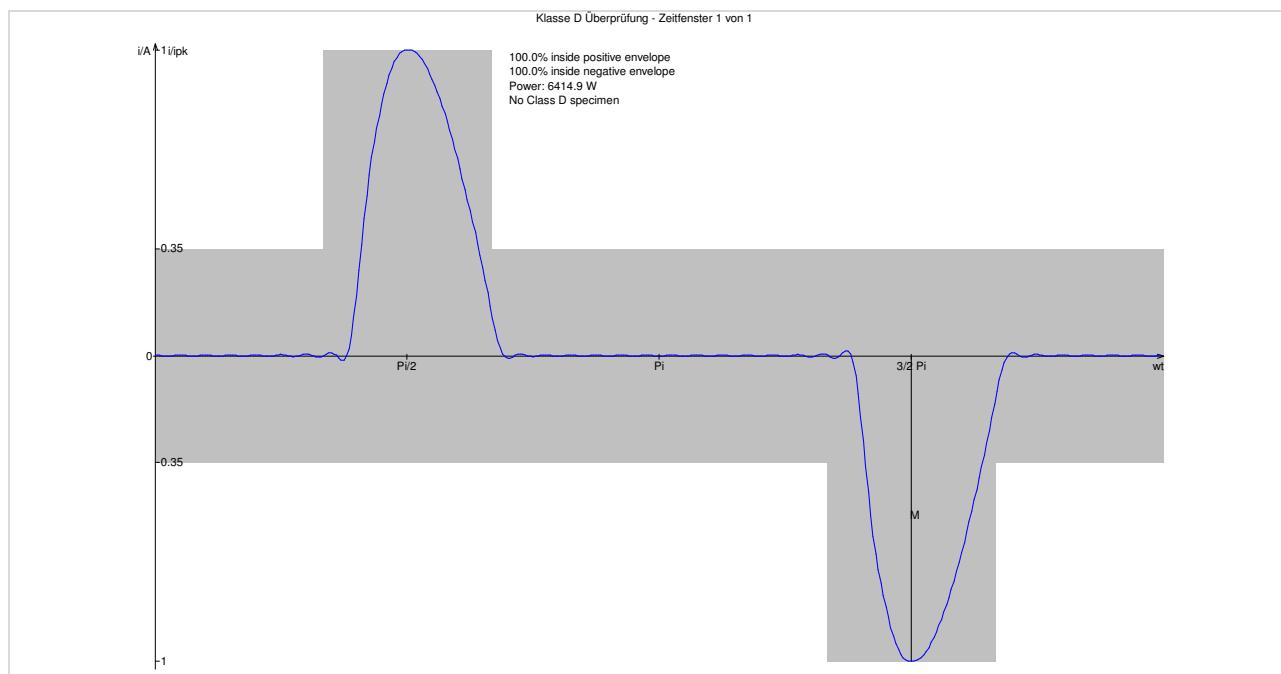
Fig. 4: Input current ( $41A_{rms}/106A_p$ ) of the EUT
