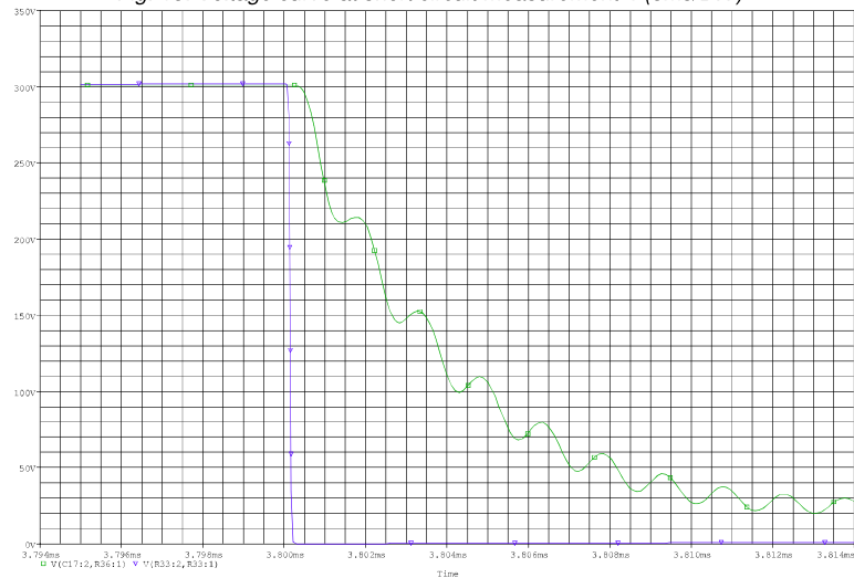
Fig. 14: Voltage curve at short circuit measurement 4 (0,5μs/DIV)
