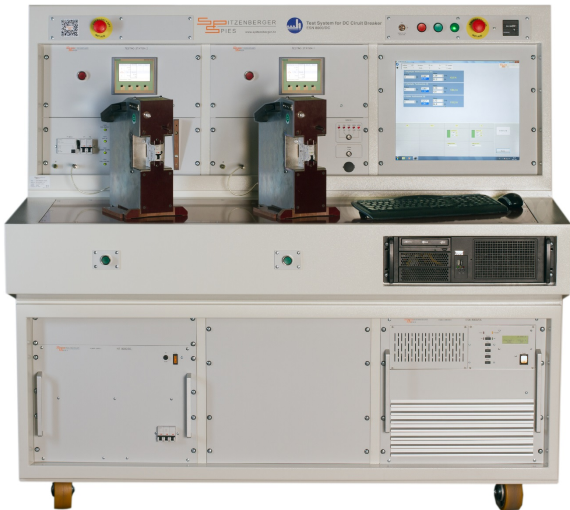
Test bench for DC circuit breakers
