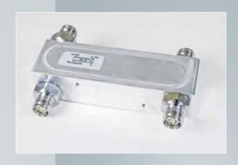
All couplers are equipped with 4.3-10 female connectors and support IP68 as degree of protection (mated). They support 500 W power rating and frequency range from 694 - 2700 MHz.
