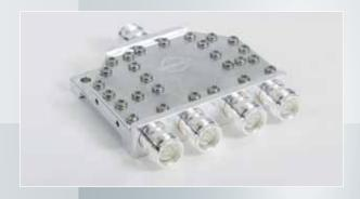
All splitters are equipped with 4.3-10 female connectors and support IP62 as degree of protection (mated). They support 250 W power rating and frequency range from 694 - 2700 MHz.
