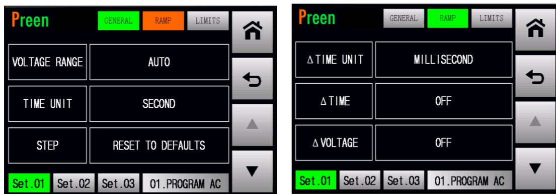
Figure 5.13 Enter into the RAMP subpage
