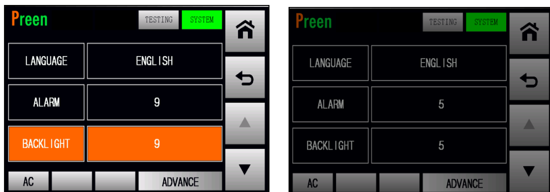
Figure 3.37 Set the backlight level from 9 to 5
