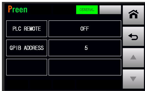
Figure 3.43 GENERAL subpage with the GPIB interface
