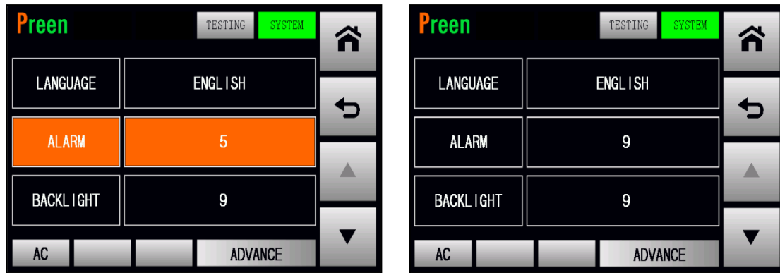
Figure 3.36 Set the alarm volume from 5 to 9
