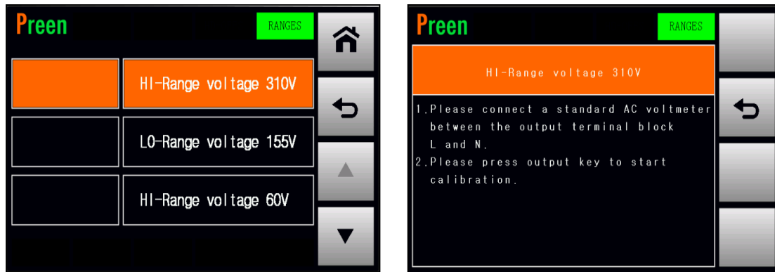
Figure 4.5 Enter into the page which calibrates the HI-Range voltage 310V
