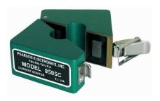
Sensitivity  $1 \text{ V/A} \pm 1\%$  Output resistance  $50 \Omega$  Maximum peak current 500 A Maximum rms current 5 A
