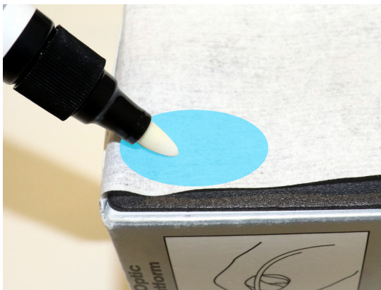
Step 3: Moisten one corner of the cleaning wipe using the fiber-optic cleaning pen or IPA pipette.
