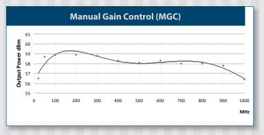
found in your typical high power RF amplifier. The amp is run in an open loop mode where the output power vs frequency changes due to device non-linearity and variations of temperature. With this mode you can take advantage of the gain peaks to get the most output power available if you are working in the associated frequency range.
