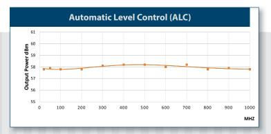
mode allows the user to command the amplifier output to a specified power level rather than adjusting the exciter to a certain power level to achieve the desired output. The output power is set either through the front panel or as a SCPI command via the LAN port . Wouldn't you rather command the amplifier to your desired output power rather than build your own feedback loop to control the exciter?
