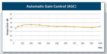
AGC mode enables internal feedback to automatically fix the gain to the level you set so the amplifier gain remains flat across the broadband range of the amplifier. This mode simplifies your system design or test setup with benefits including:
