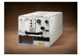
Model VZA2791J1 150 W CW power amplifier for EMI/EMC testing applications
