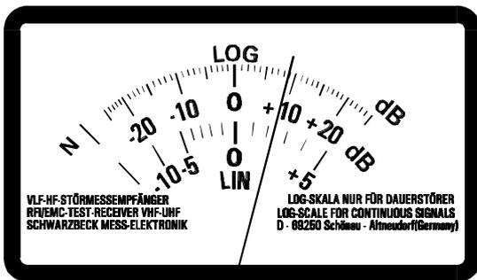
The meter uses the classic 0 dB centre of meter scaling for safe measurement without interpretation.
