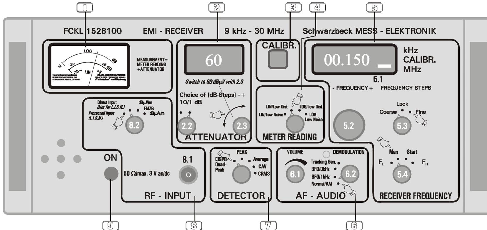
The front panel is divided into 8 areas, which unite important controls and displays.
