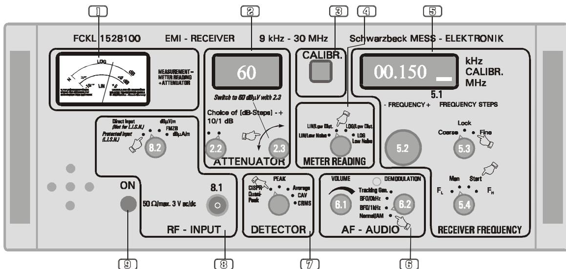
B) Set steps to Fine with (5.3), which is recommended by the arrow. This means that there are 10 Hz-steps in band A and 1 kHz-steps in band B.
