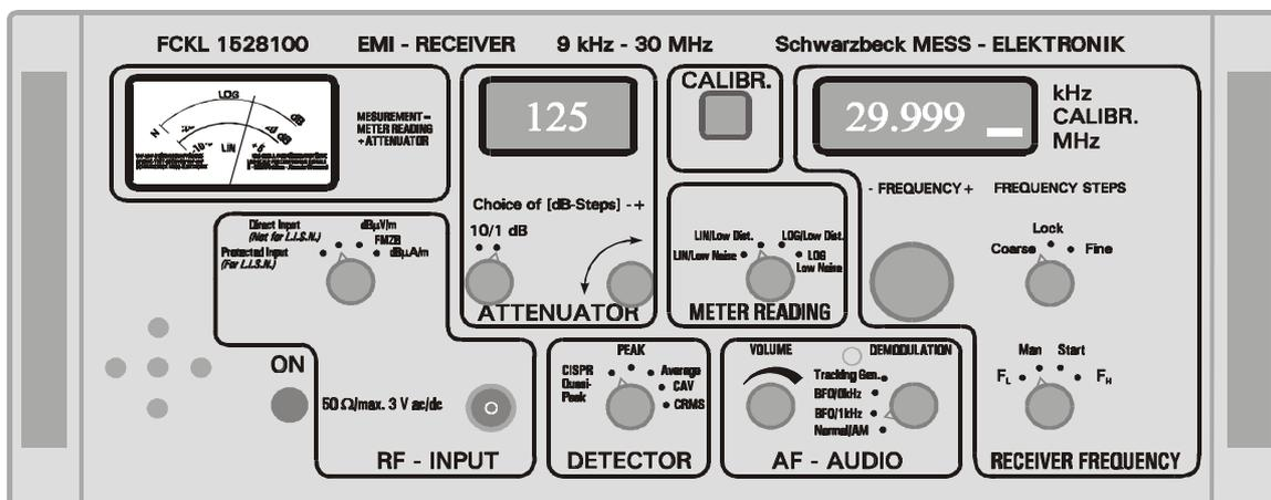
Interference measuring receiver for front panel operation with or without
