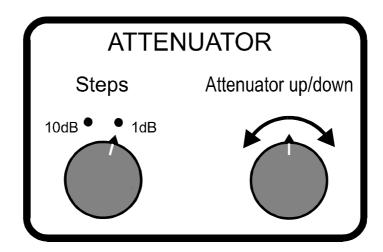
The field Attenuator serves for the control of the step attenuator.
