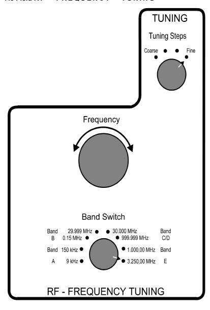
Switch TUNING selects the digit to tune the frequency when rotating the rotary encoder.
