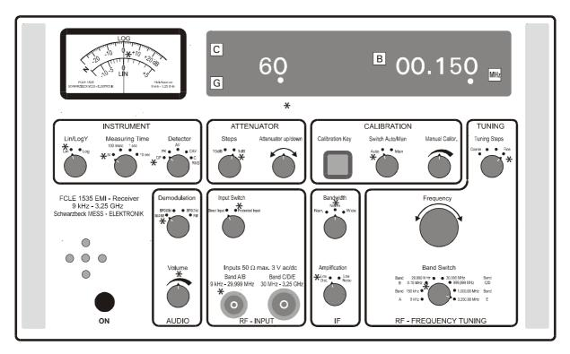
Step 2: Connect the r.f.- output of the l.i.s.n. to the receiver's left r.f. - input (bnc).
