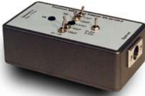
Common mode test adapter MGA_B1 according to Fig. B.1 (EN 55103-2)
