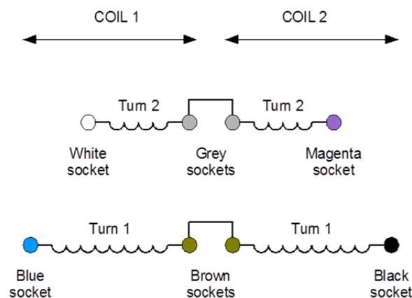
If the output of a power amplifier is connected to the "blue" and "black" jacks, a Helmholtz coil with a high coil factor is available, ideal for generating high field strengths at low frequencies where the coil inductance is not yet important.
