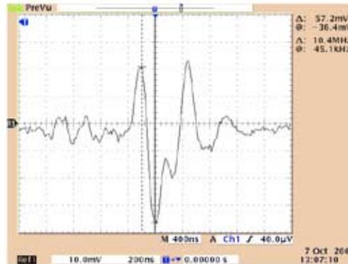
Figure 2a. Current in GBB (gold ball bonding) Tool (peak current is 182mA)
