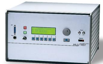
The high-voltage impulse generator PG 10-1000 generates standard impulse voltages with waveforms  $1.2/50~\mu s$  and  $10/700~\mu s$ . Output voltage is adjustable between 0.5~kV and 10~kV. The polarity of the output voltage is selectable. Positive, negative or alternating polarity of the output voltage can be preselected.
