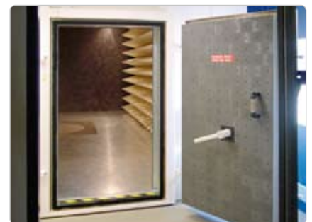
Door with ferrite absorbers
