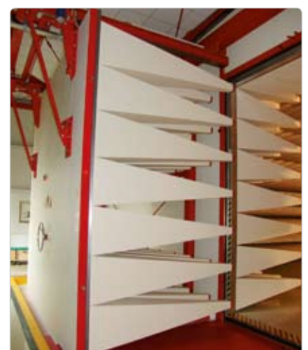
Sliding door with pyramid absorbers
