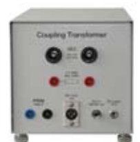
Coupling transformer CT 2.5/50 AC with differential amplifier
